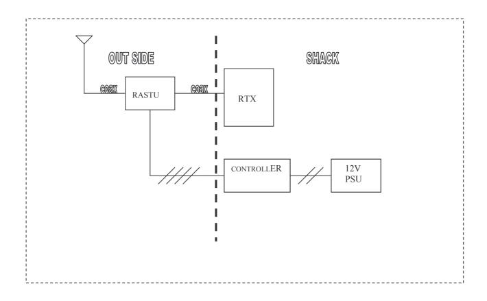
With the aim to allow RASTU working with any commercial RTX, as well with home-built radio transmitters, the CONTROLLER provides a closed contact criteria to be possibly wired towards any generic RTX, in order, for the latter, to revert automatically a "C.W. Low Power (5-20 W)" condition during the required tuning time.
